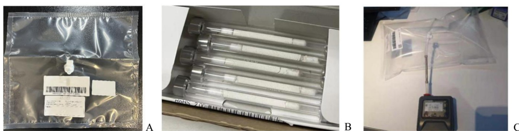
A: Tedlar sampling bag; B: Thermal desorption tube; C: Use the sampling pump to transfer the gas from the Tedlar sampling bag to the thermal desorption tube.
