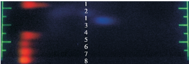
图 7 琼脂糖凝胶电泳照片 Fig. 7 The photo of agarose gel electrophoresis 1: QD-PEG; 2: PEG-FA; 3: PEG; 4: FA; 5: QD-PEG-FA; 6: QD-PEG+FA; 7: QD-PEG; 8: QD. QD was Cd Te/CdS.
